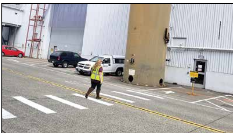
AFTER: A newly painted white crosswalk leads directly to the pedestrian door for safe pedestrian passage.
