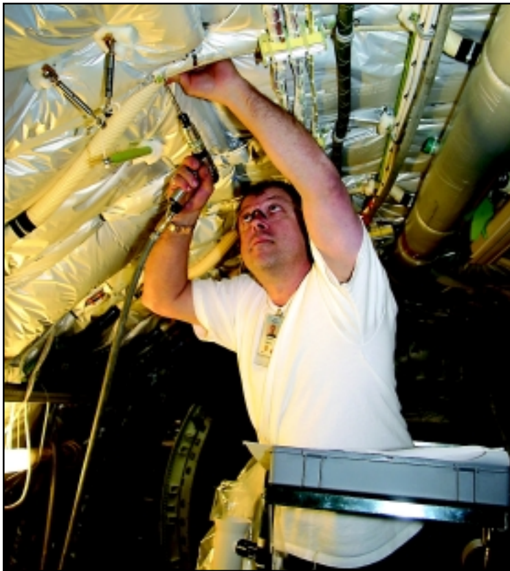
Steve Selby installs the tubing for the 737 air conditioning system. The crew came up with innovations and process changes that reduced the time to perform their work package by 90 percent.
