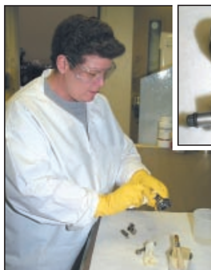
Linda Relford removes green seal from the clevis using 'paint lift.'
