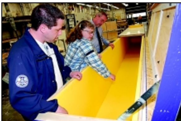
Connie Nichols (center) explains to Scott Donohoe (l) and Business Rep Tommy Wilson how new shipping boxes eliminate twisting at awkward angles to load/unload parts.
