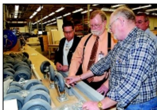
Steward Ken 'Red' Jordan (r) explains to Steward Scott Donohoe (l) and Business Rep Joe Crockett that by assembling the wheel and brake locks in tooling, the price for the wheels was cut in half.
