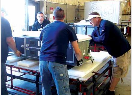
Using the previous cart to move closets required four to six members bending in awkward positions to lift the closets. Often one member would walk backwards across the platform creating a huge safety hazard.
