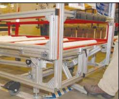
Above: the foot lever that locks the cart in place and raises the rollers to unload the closets is just one of the design innovations.
