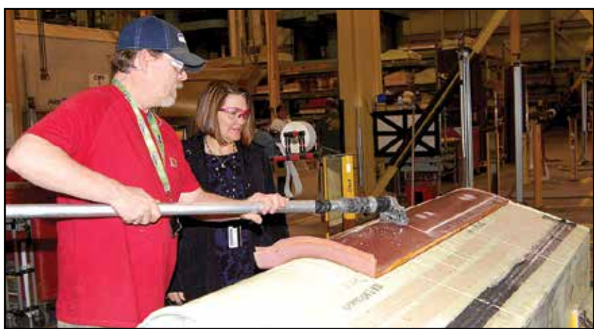
Patrick Tingley shows Business Rep Grace Holland the new system. The union helped ensure an adequate vacuum system was installed for the 5-axis machines after nearly every member in the shop suffered strains and sprains trying to do their job with an inadequate system.
