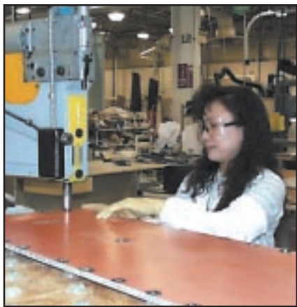
Toanh To works on a floor panel for Boeing planes at the Spokane Triumph Composite Systems.
