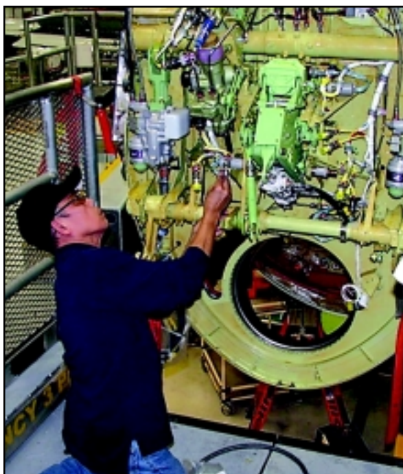
In Renton, 751 member Catalino Antes works on wiring for the aft section of the P-8A Poseidon airplane.
