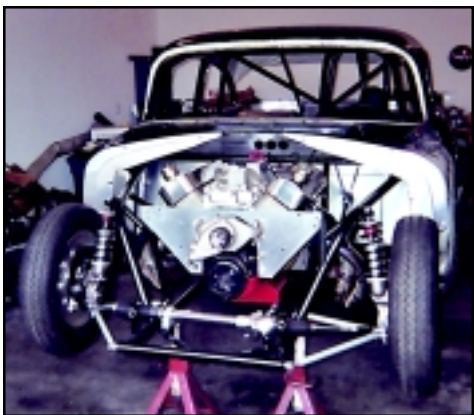
John cut and notched the parts, welded the tube to form the chassis and fabricated the sheet metal.
