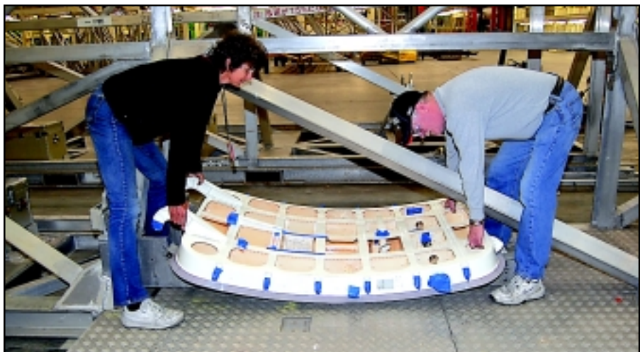
751 members Carole Lamoureux and Steve Benson show how employees used to lift 767 doors before an innovative lift tool was made. Due to extensive crossbeams on the shipping tool, there was no safe way to move the door.
