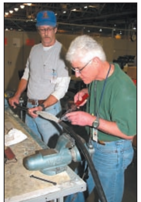
In a hands-on lab, James Cox (l) and Ralph Slansky solder a cable after completing a splice to a medium-voltage cable.
