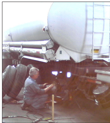
Steward Danny Wohl performs a brake overhaul.
