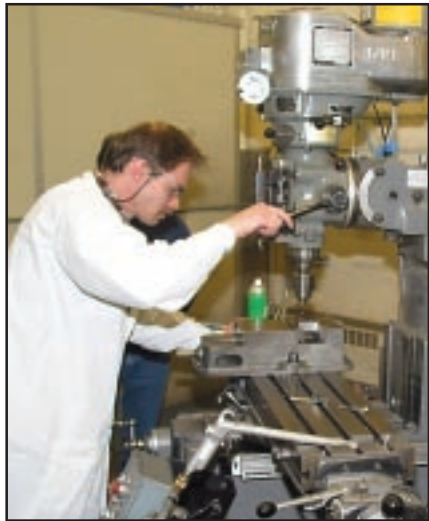
Martin Schmidt performs a drill and tap operation on a mill, as part of a peer training class.
