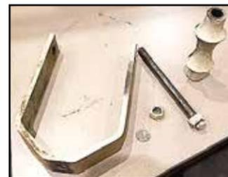
The 1-pound bolt that fell and the 6.8 pound bracket and roller it had been attached to, which was only held in place by friction after the bolt worked loose and fell.
