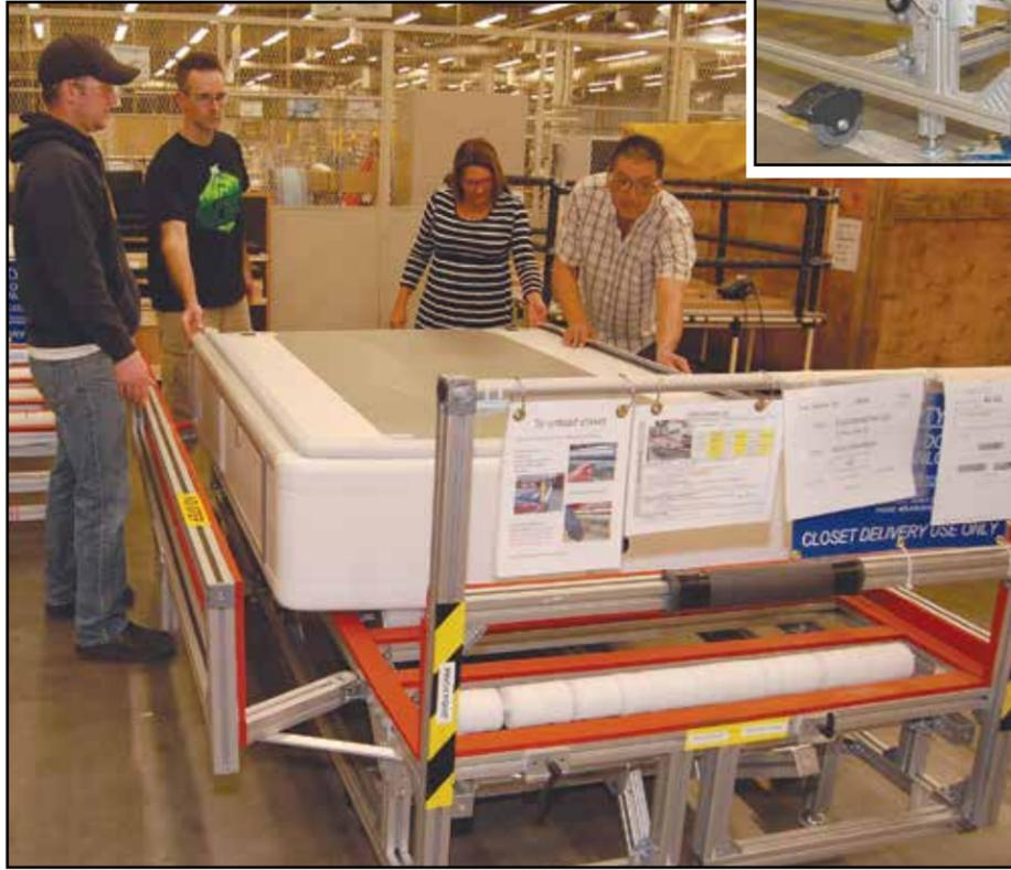
Above: the foot lever that locks the cart in place and raises the rollers to unload the closets is just one of the design innovations.
