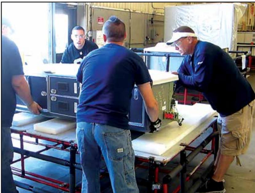
Using the previous cart to move closets required four to six members bending in awkward positions to lift the closets. Often one member would walk backwards across the platform creating a huge safety hazard.
